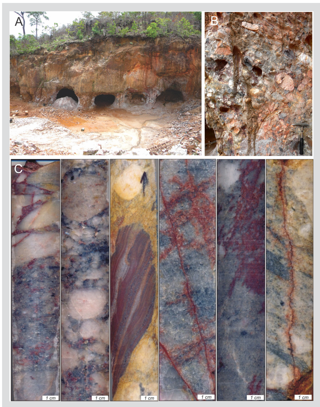
FIGURE 5 - Images of metaconglomerates of the Castelo de Sonhos deposit. (A) General view of an artisanal mining pit. (B) Closer view of the clast-supported metaconglomerate, with pebbles of variable shapes and sizes. (C) Drill cores showing, from left to right: impregnation of secondary iron oxides in the matrix and in fractures; clast-supported metaconglomerate; clast of banded iron formation; fractures coated by secondary iron oxides; strong impregnation of the matrix with secondary iron oxides; fracture coated by secondary iron oxides cutting across matrix and clasts.
