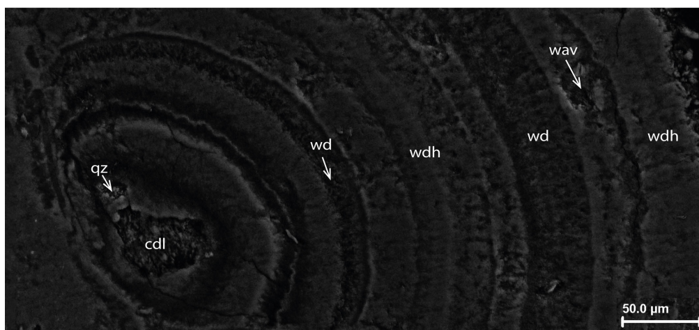
Figure 7: Colloform crandallite (cdl) nodule precipitated around relic quartz (qz). In the darker zones, millisite (mill) formed, intercalated with woodhouseite (wdh), and mitridatite (mit) occurs at the rim along with wavellite (wav) inclusions.
