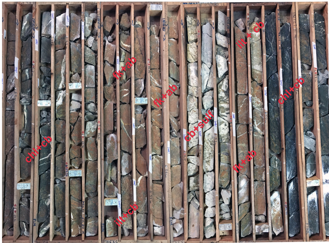
FIGURE 11. Core section from drill-hole SB-09 at the Santa Bárbara Deposit, Between Depths of 45m and 65m (Left to Right). This section shows pervasive potassic and albitic alteration (red and pink colors), overlaid by carbonate fissure zones (white) and illite-rich areas (beige), along with pervasive chloritization (dark gray). Abbreviations: fk+ab: feldspar and albite alteration; ilt+cb: illite and carbonate alteration; cb+sulf: sulfide-bearing carbonate alteration.
