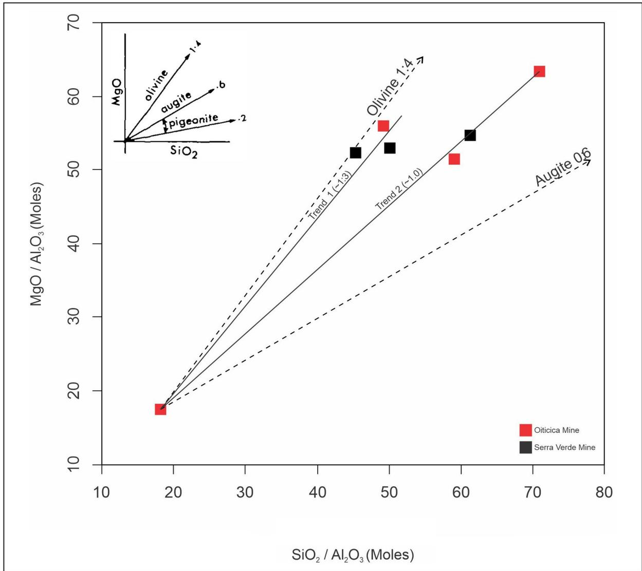
FIGURE 6. MgO/Al<sub>2</sub>O<sub>3</sub> vs. SiO<sub>2</sub>/Al<sub>2</sub>O<sub>3</sub> Diagram (Pearce 1968, 1970) for the studied serpentinites. The arrows indicate the fractionation paths of olivine, augite, and pigeonite, while the lines represent the two trends formed by the analyzed samples.
