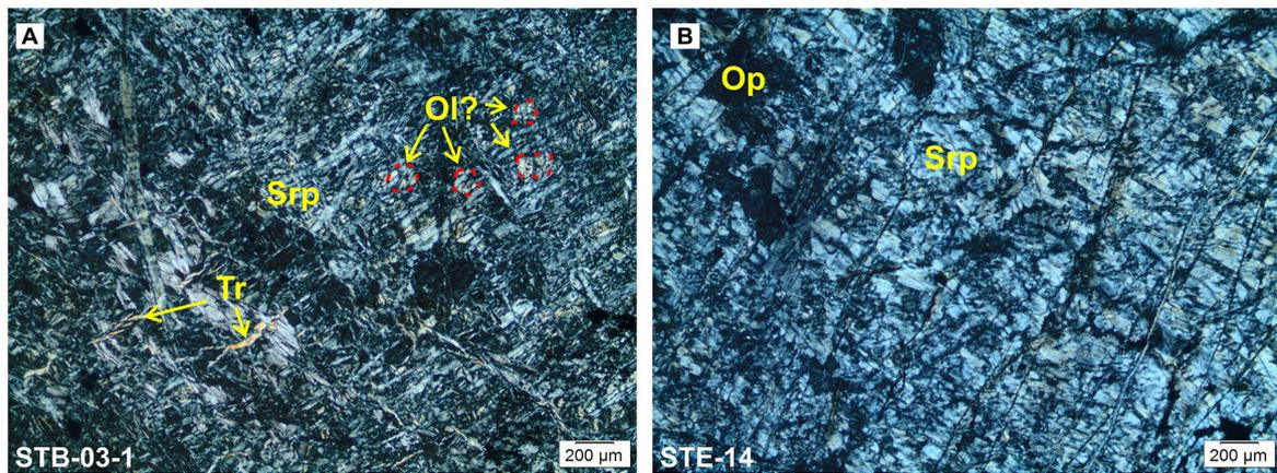
FIGURE 4. A. Photomicrography of serpentinite: A. Photomicrograph of serpentinite from the Oiticica Mine, transmitted light, N X; B. Photomicrograph of serpentinite from the Serra Verde Mine, transmitted light, N X. Mineral annotations: Srp = Serpentine, Op = Magnetite, Tr = Tremolite, Ol = Olivine.
