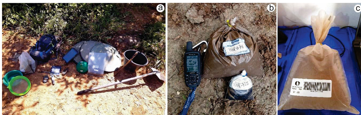
FIGURE 4. Materials used to collect geochemical samples (a) and examples of samples (b) collected from active stream sediment and heavy mineral concentrate (GeoSGB). Subsequently, the samples are weighed and identified with barcodes (c).
