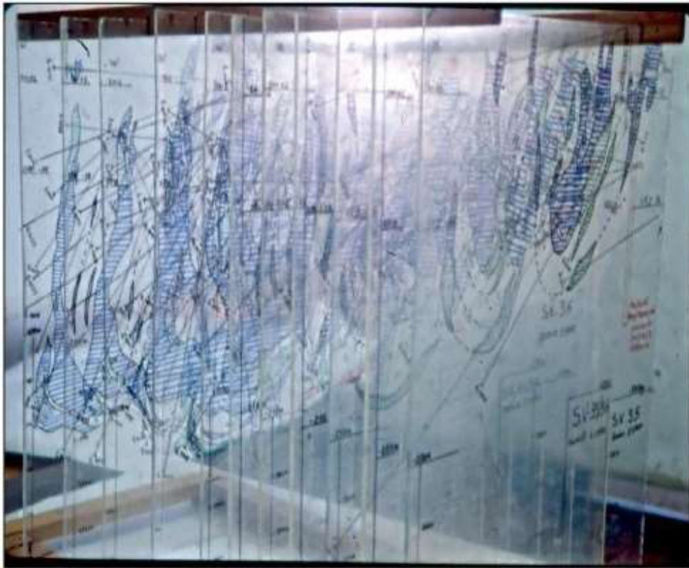
Figure A2-7: A 3-D translucent view of the Caraíba F_3 synform on space, based in the drawing of the most updated vertical geological sections across the Caraíba orebody, obtained on 1998, on transparent sheets of plastic material. Nothe the South-plunging fold hinge.
