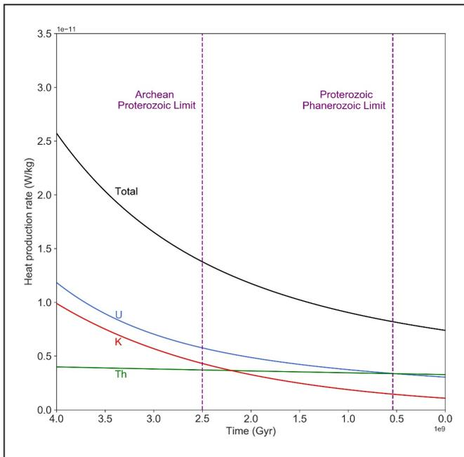
**FIGURE 1.** Difference in heat flow over time for radioactive elements. The graph shows the radiogenic heat emitted by K and U and Th decay series on the vertical axis. The horizontal axis shows the time (Earth Age) from 4.0 Ga onwards highlighting the decay curve of the U series in relation to that of Th, which for this time scale is shown as an almost straight line, since the half-life of  $^{232}\text{Th}$  is three times larger (modified from Turcotte and Schubert, 2014).
